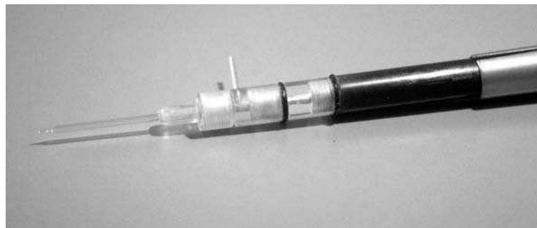
Fig. 3-13 A glass micropipette in a holder. The thin side tube allows to apply pressure (tracer injection) or suction (membrane patch attachment).
