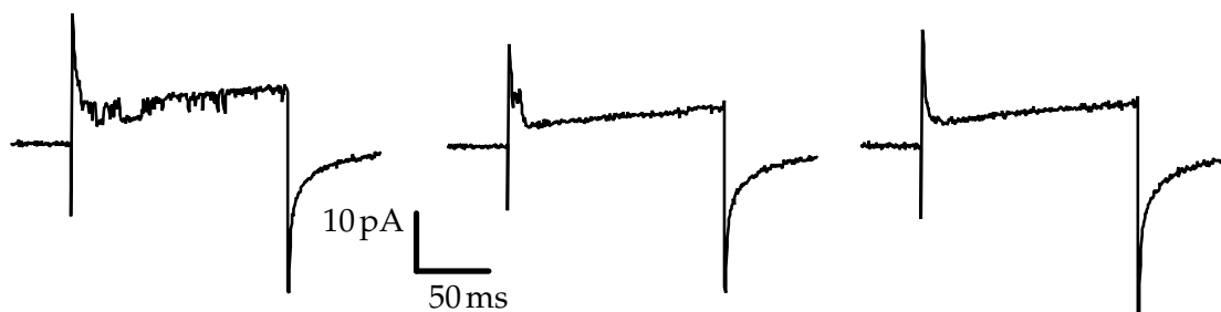
Fig. 4-58 Capacitive current peaks that hamper channel current measurement.
