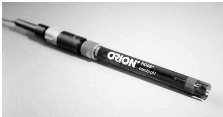
Fig. 3-10 A pH electrode with built-in reference (AgCl) electrode.
