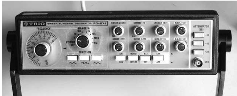
Fig. 2-39 A practical form of function generator. The left knob and switches control waveform and frequency, the rightmost knobs control the amplitude and DC offset. The middle controls are for creating sweeps, asymmetric waveforms, etc.
