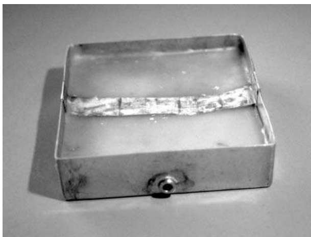
Fig. 3-15 A silver strip ground, electrode in an insect preparation tray.
